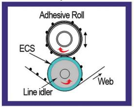
TCS web cleaner: Pre-sheeted Adhesive Roll (Patent Pending) with automatic actuation system mounted against a line roller fitted with an ECS Elastomer Cleaning Sleeve.
