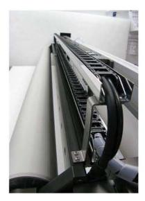
When roll cleaning is required the unit switches to washing mode on a user programmable timing cycle. The TSRR roll connects to the integral drive motor and is rotated whilst being cleaned by an operator (semi-automatic) or a traversing wipe (fully automatic). Slide pull-out of the roll is also an option if side access is required.
